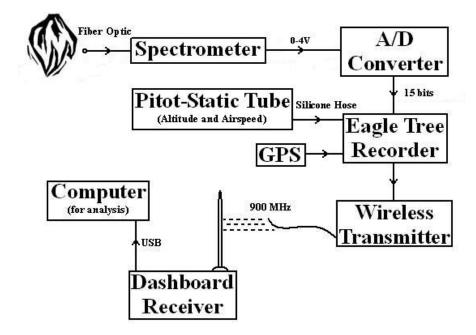
Figure 4.7 Schematic of microcontroller subsystem.
