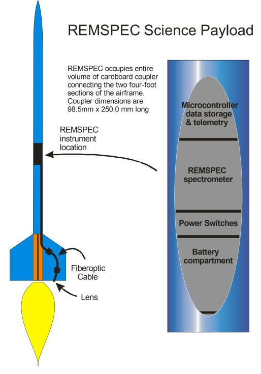
Figure 4.1 Schematic showing REMSPEC location and fiber optic cable placement.
