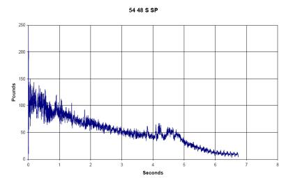
Figure 3.5: K-265SP Thrust Curve.
